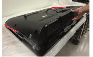
D Hold Power Supply Cord while lifting up Rear Cover, then pass Power Supply Cord through Rear Cover opening
