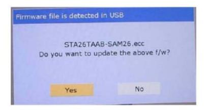
The firmware upgrade window will appear next.Do not disconnect AC plug or turn off TV while updating.
